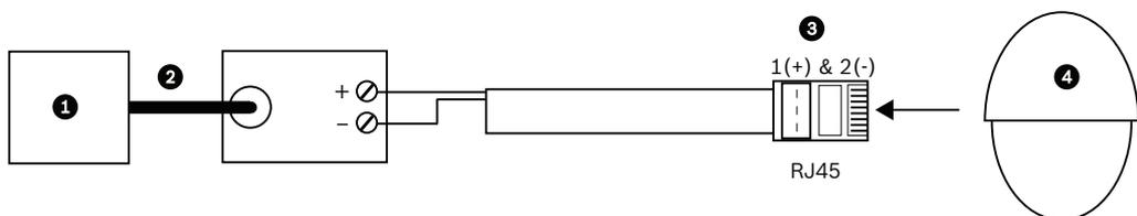
**Figure 3.1** Video and Control over UTP
