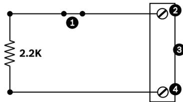
**Figure 4.2** N.C.S. - Normally Closed Supervised Connections
