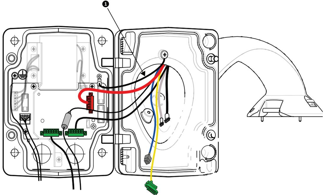
Figure 2.11 Analog AutoDome: Pendant Arm connections to Power Supply Box
