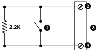
**Figure 4.1** N.O.S. - Normally Open Supervised Connections
