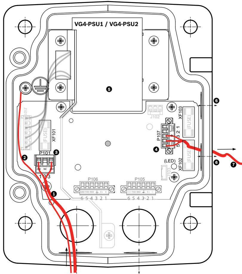
**Figure 2.6** VG4-PSU1/VG4-PSU2 Power Supply Box
