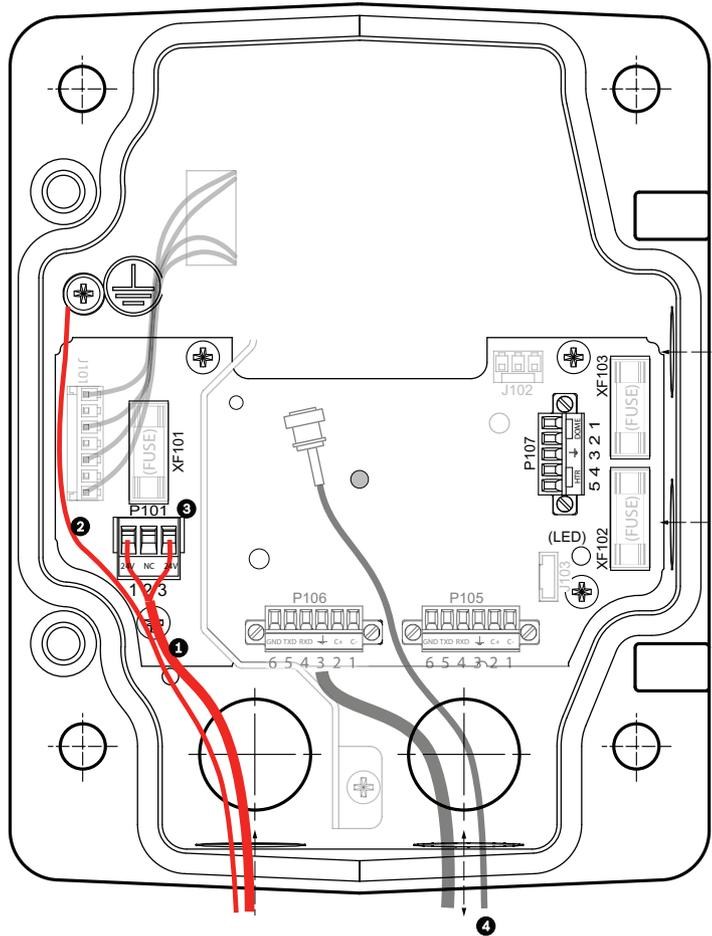
**Figure 2.9** VG4-PA0 Power Supply Box
