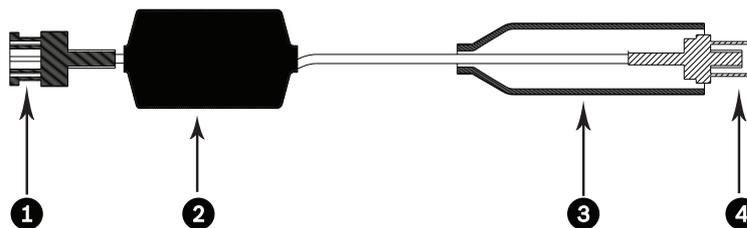
**Figure 2.2** Coaxial cable with ferrite
