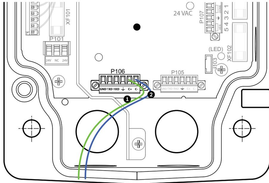
**Figure 3.8** Detail of P106 Connections
