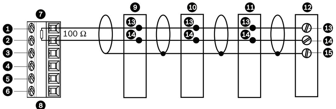
**Figure 3.3** Connections for a Daisy Chain Configuration
