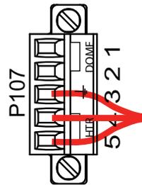
**Figure 2.8** Outgoing 24 VAC power supply
