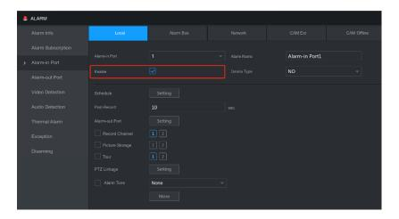
**#Step2:** Enable the Mobile Push Notification in advance, and select the "off" as disarming status, so once you tragger the alarm input 1, the disarming status will change to "On", then the NVR will stop send the push notification to DMSS app.
