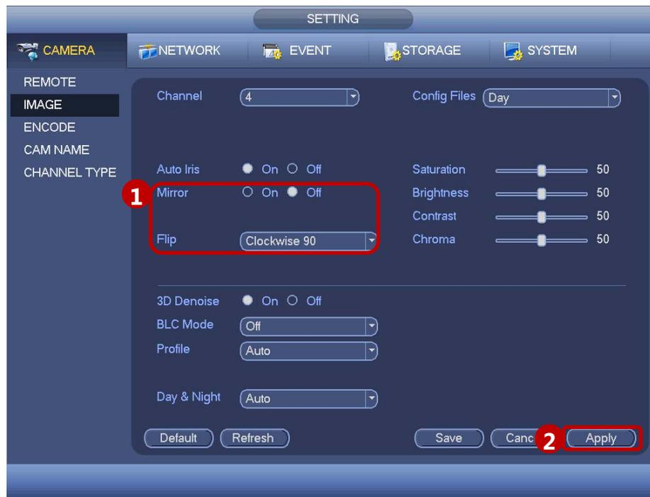
**Corridor mode**(for **IP cameras only**): flip the image to make the image suitable for surveilling corridor.
