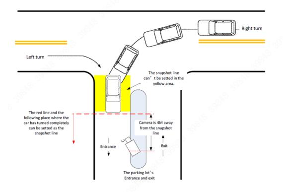
During snapshot, make sure the vehicle has complete turn and being moving straight.
