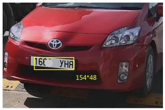
Make sure the pixel size of the plate at the snapshot position is within certain range below:
