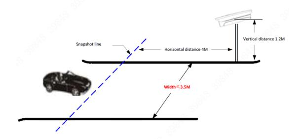
Camera installation height is 1.2m, lane width is smaller than 3.5m (If the lane is too wide, you can place isolation pile to guide vehicle flows), the horizontal distance from camera to snapshot position is 4m.
