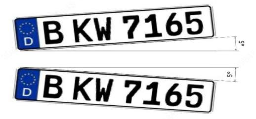
Make sure plate inclination angle is always smaller than  $5^{\circ}$ .
