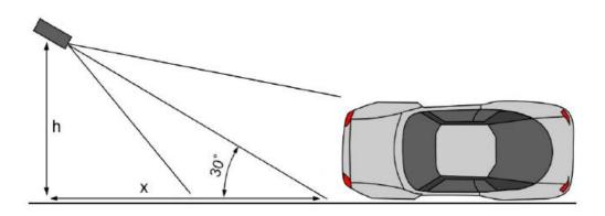
The angle between camera lens and the farther lane border shall be smaller than  $30^{\circ}$ . The camera is at a distance of h meters away from the further side of lane, and snapshot distance is x meters,  $x \ge 1.7h$ .
