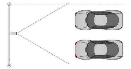
During front-installation, a camera can monitor 1 lane, only ITC237-PU1B can monitor 2 lanes when the installation height is over 3 meters. When a camera is installed at center of a lane, it monitors this lane only. When a camera is installed at border between 2 lanes, it monitors these 2 lanes at the same time.
