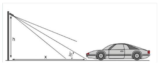
No matter front-installation or side-installation, the angle between camera lens and the ground shall be smaller than  $30^\circ$ .
