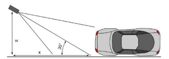
At side-installation, a camera can monitor 1 lane, only ITC237-PU1B can monitor 2 lanes when the installation height over 3 meters, The angle between camera lens and the farther lane border shall be smaller than  $30^\circ$ .
